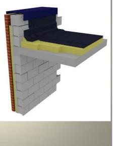
Remove capping, flashings and roof coverings to expose **CMU** wall and roof insulation
