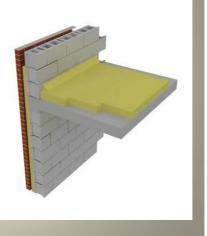
Now add rigid insulation to the rear and top of the parapet as well as the cavity if possible
