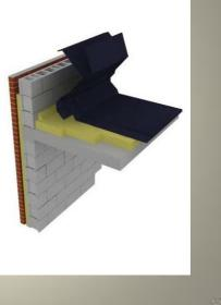
Remove capping, flashings and roof coverings to expose CMU wall and roof insulation
